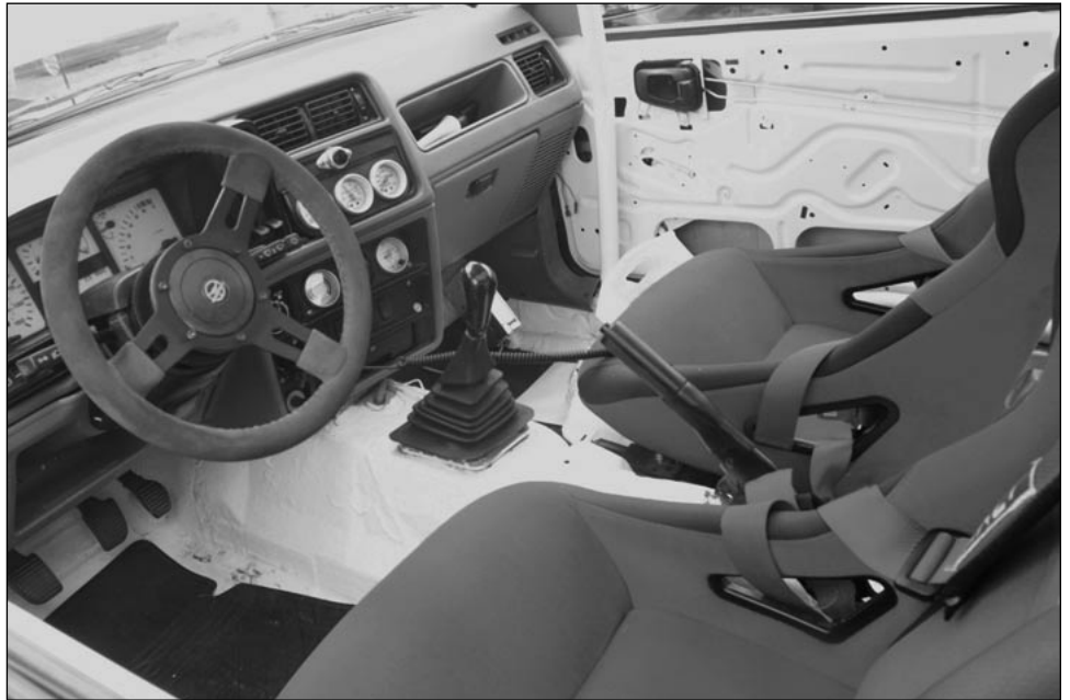
Stripped interior (right) in Mohammed Saoik's XR. Note extra gauges, white gauge faces, matching red custom steering wheel, four-point seatbelt harnesses.
