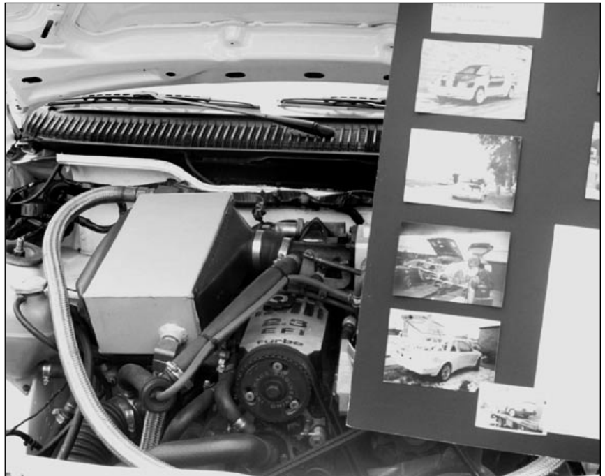
Water-to-air intercooler highlights Stuart Matthews' highly modified XR engine bay, a WRC replica XR, painted green and white. Exterior photo on back page.
